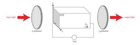
It is composed by two polarizers in cross configuration, and a KDP crystal with optical axis along z (z-cut) and voltage applied on the input/output facets of the crystal.
