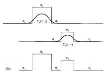
It is composed of two waveguides separated by a finite distance. In the following analysis we will assume for simplicity that the waveguides are monomodal and support a fundamental  $TE_0$  modes, whose electric field  $E_a$ and  $E_b$  is sketched in the figure on the left.
