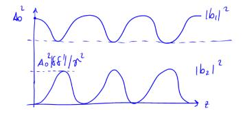
The maximum power transferred on the waveguide 2 is  $P_m = \frac{|\delta|^2}{\gamma^2}$ .
