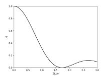
By adjusting the mismatch  $\Delta$  to  $\Delta = \frac{\pi\sqrt{3}}{L_c}$ , we inhibit transfer of energy to the other waveguide and the device maintains the output on the same channel (bar-state). By piloting the device from  $\Delta = 0$ (cross-state) to  $\Delta = \frac{\pi\sqrt{3}}{L_c}$  (bar-state), the coupler operates as an integrated switch.
