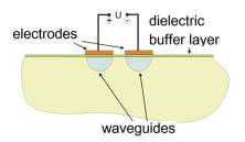
The main idea is to use control the refractive index of one arm with a nonlinear effect such as, e.g., the electro-optic effect. This, in turn, will adjust the propagation constant  $\beta$  of one mode controllably, allowing fine tune of the resulting mismatch term  $\Delta$ .
